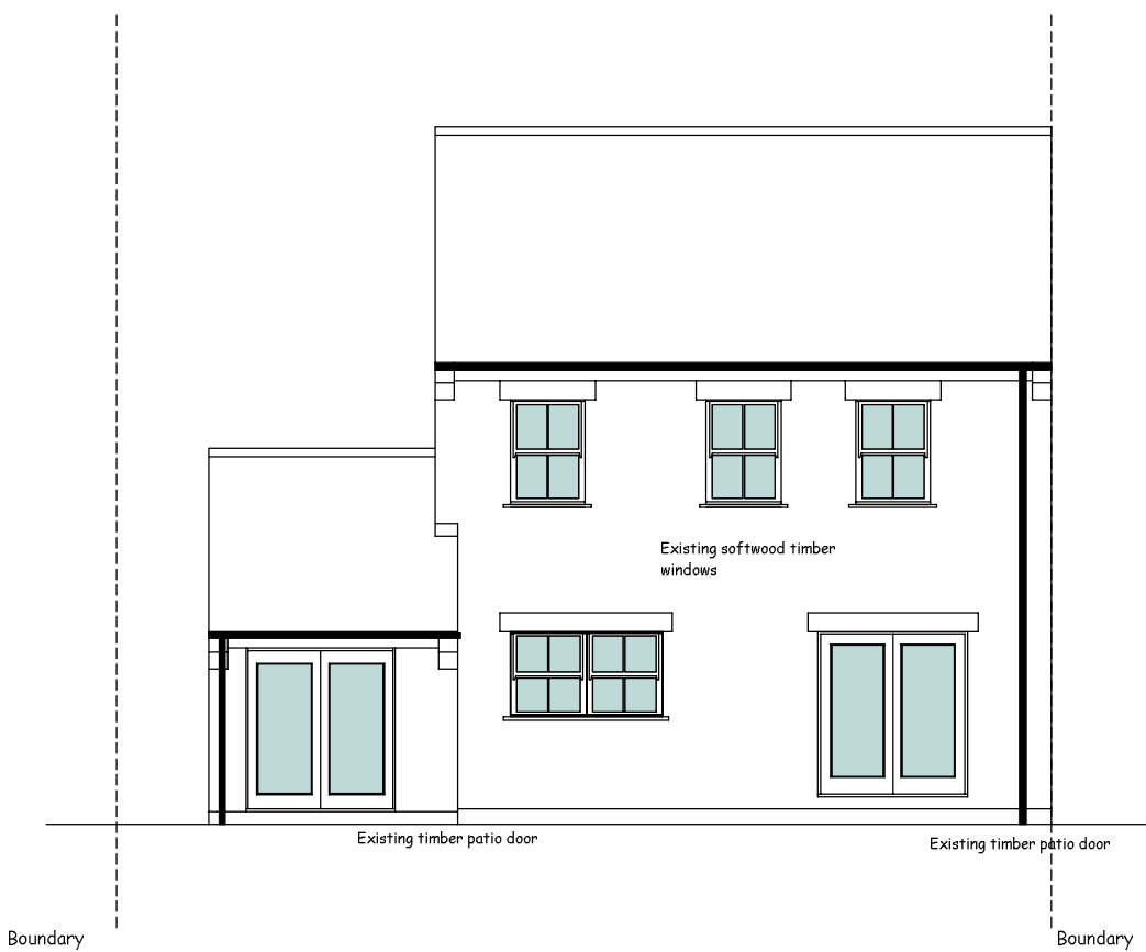
Existing Rear Elevation
